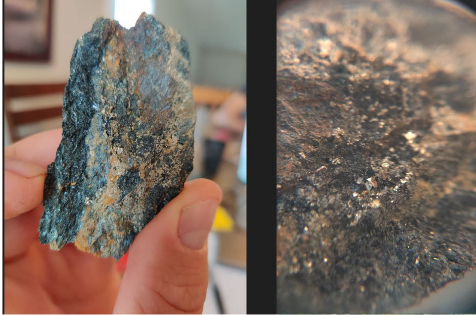
Figure 8: Sample 110521, sheared gabbro with pinch and swell qtz veining. 15% pyrite and 2% chalcopyrite.
