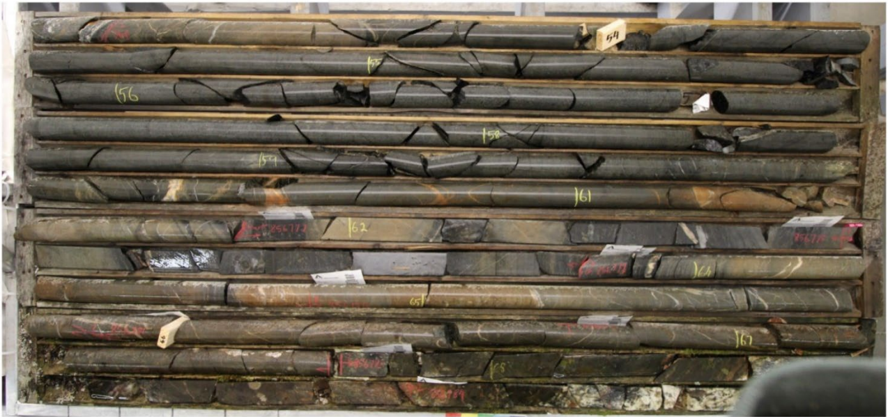
Figure 11: BZW0805 Dry(above) and Wet(below) Drill Core Box 13-16
