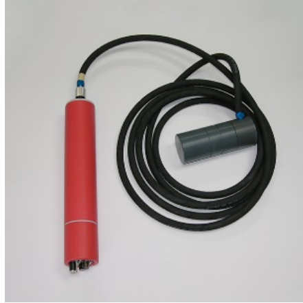
Figure 7 – Scintrex CS-3 magnetometer sensor, cable, and electronics.
