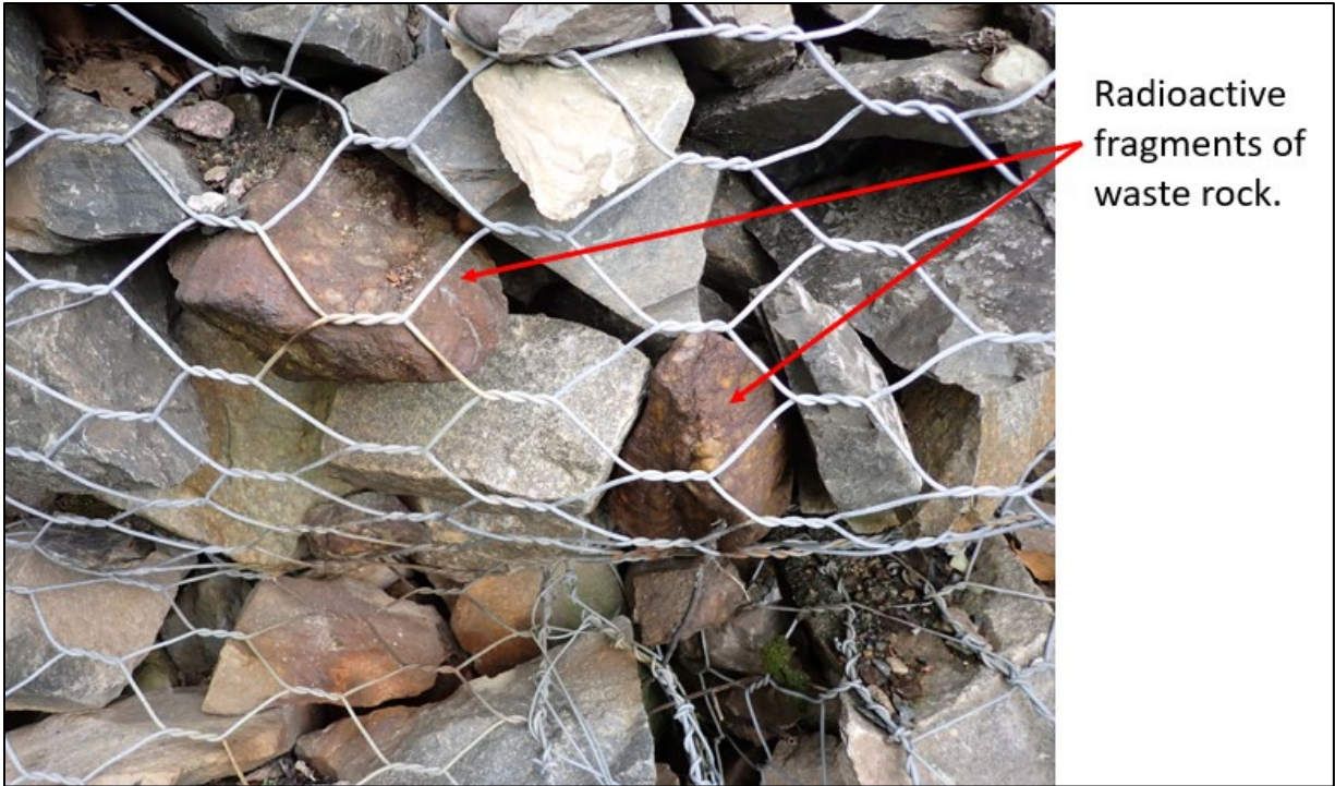
Figure 16: Radioactive fragments of waste rock confined with a wire mesh; station 22-LAH-033.
