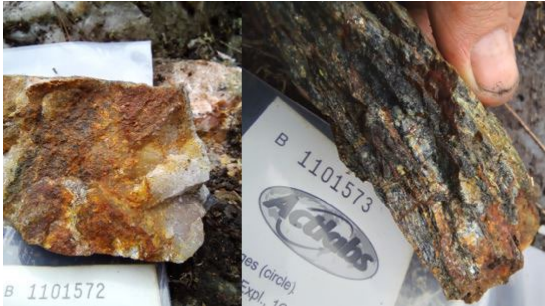
Figure 6: Mineralized quartz vein and sheared mafic volcanics discovered at the location of the Anglehart Showing
