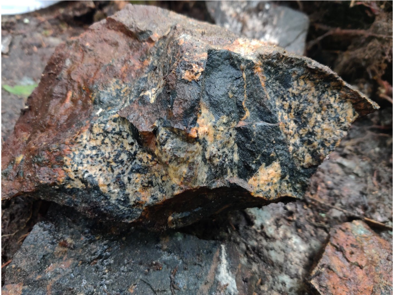
Figure 7: Fractured, silicified mafic volcanic with 2% sulfides. (Sample 1101591)
