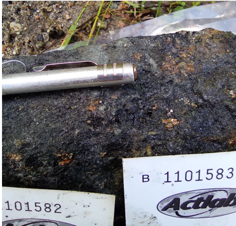
Figure 8: Strongly mineralized biotite-pyroxenite with 2-5% pyrite and chalcopyrite taken from the area of 16JW584 (Samples 1101582 and 1101583)
