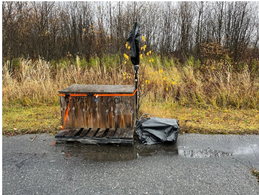
Figure 9 – Base station magnetometer used for diurnal corrections.
