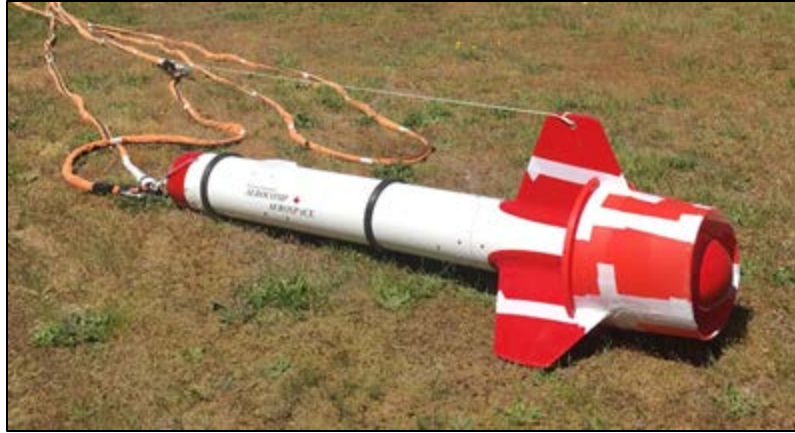
Figure 8 – Airborne magnetometer housing with tow cable.
