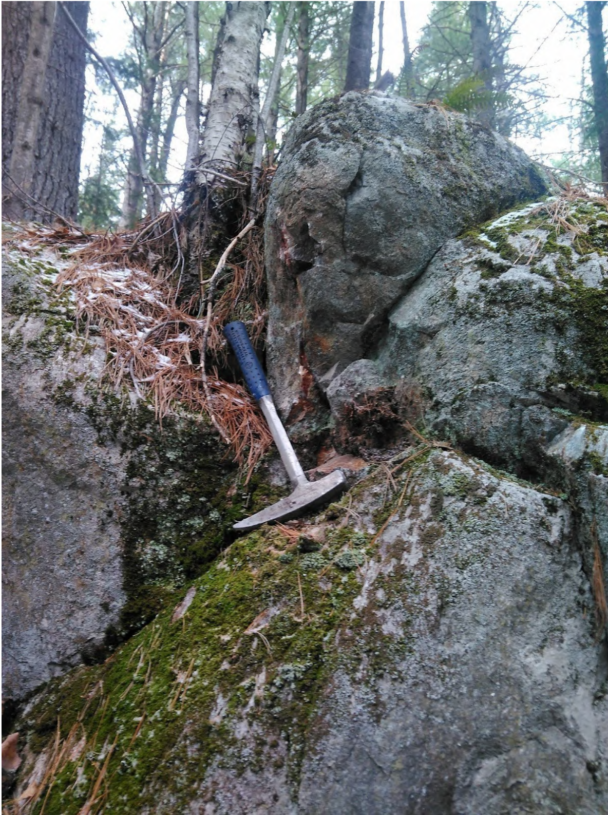
Photo of typical grey monzonite. The 2-centimeter rusty quartz vein above the rock hammer handle was sampled and submitted for gold assay.
