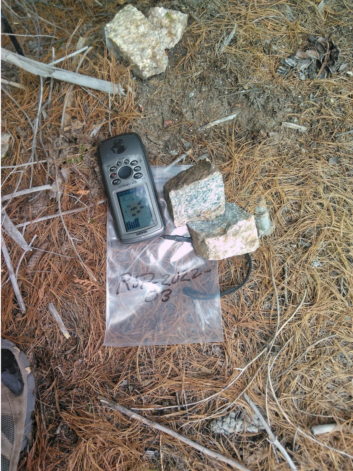
Photo showing sample RSR-2022-03 at next outcrop sampled on an eastern direction along the Red Squirrel Road. The monzonite has a 50% K-feldspar content, shown as pink swiffs within the mafic equivalent.
