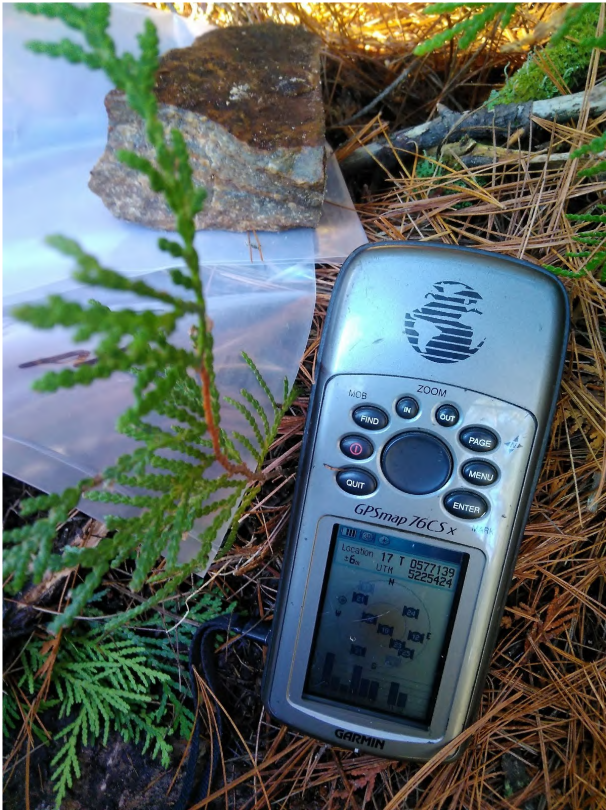
Photo shows GPS location of sample 05-21-RSR and a closeup view of the sample, showing the rusty banding and some visible pyrite crystals randomly distributed within the banding.
