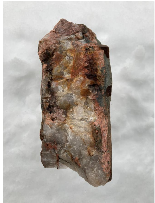
Quartz-feldspar specimen with massive sulfides visible along left edge of sample (archived as 112 LHM 302)
