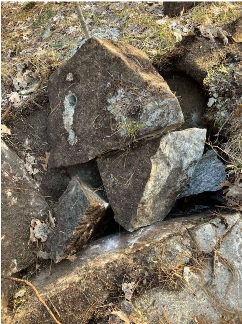
Figure #4 Blasted product – Rock fractured along foliation planes. No fly rock, large material generated
