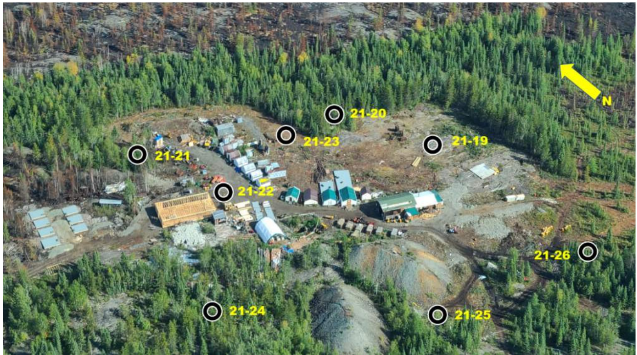
Figure 22. Collar locations for drill holes in the vicinity of the "mine area" at Lingman Lake. All holes were drilled toward the north. Note burned area at the top and left part of the photos due to RED 81.
