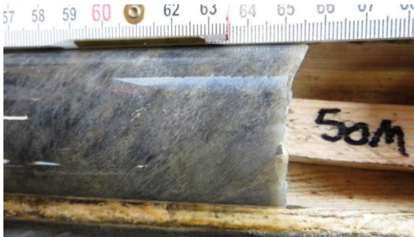
Figure 13. Altered mafic volcanic with a tuffaceous or cherty appearance form 50 m depth in hole 18-03
