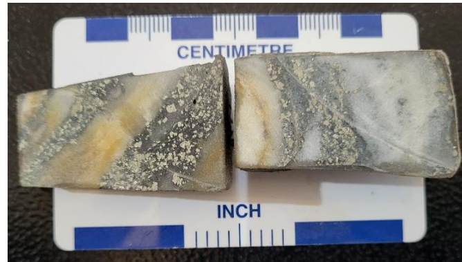
Figure 1 Images of thin section blanks illustrating the alternating quartz banding and retrogressive sulphide domains within samples A and B.
