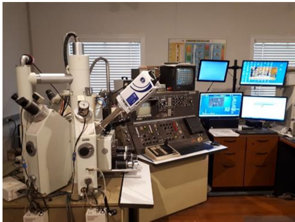
JEOL JXA-733 Superprobe equipped with an Oxford Xact EDS system housed in the Laboratory of Renaud Geological Consulting Ltd.
