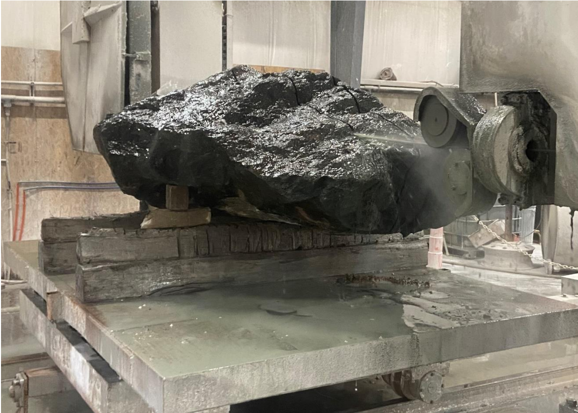
FIGURE 9 GRAY GNEISS SAMPLE UNDERGOING SLAB CUTTING FOR WEATHER DURABILITY TESTING
