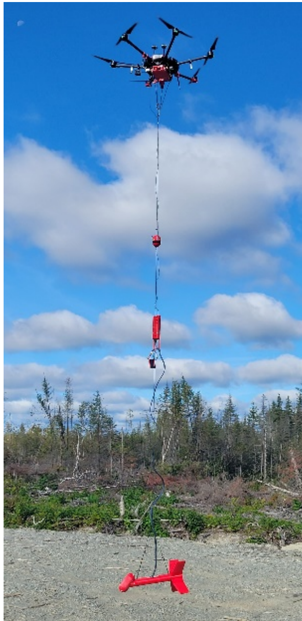
Figure 6-4: Vision 4K UAV magnetometer system configuration.
