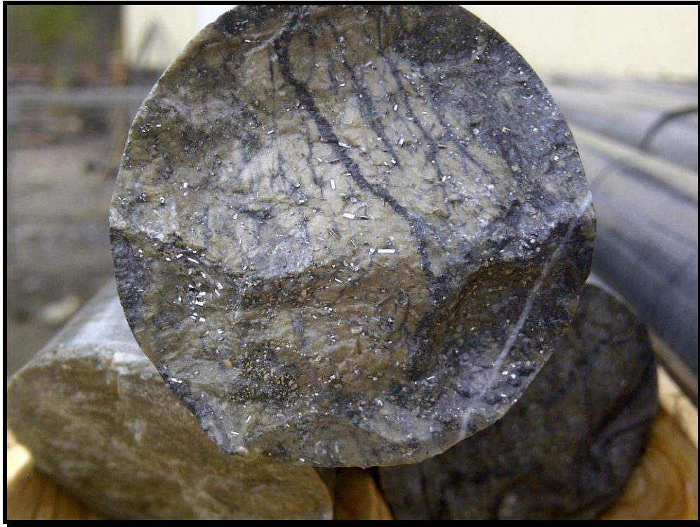
Albite alteration cut by quartz typical of South Zone with strong arsenopyrite
