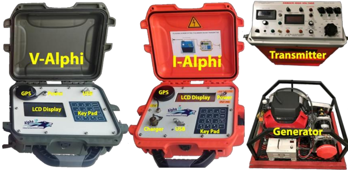
Typical Alpha IP Current Recorder and Voltage Receiver (Alphi)
