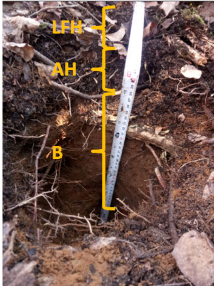
Figure 6: Photographs of small sampling hand-dug pit of sample 153940042 where mineral B-horizon soil is visible underneath 4 cm thick LFH horizon, 4 cm thick decomposed organic matter Ah and 1 cm thick eluviated horizon Ae. Sampling depth of this hole was 18 cm.
