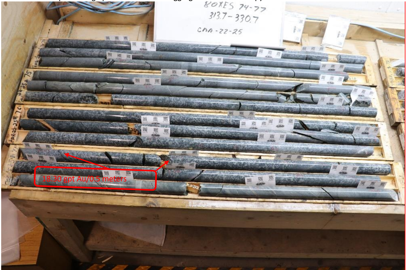
Figure 5: Drill core intercept in CAR-22-25 showing several quartz sulphide veins cutting through feldspar porphyry.
