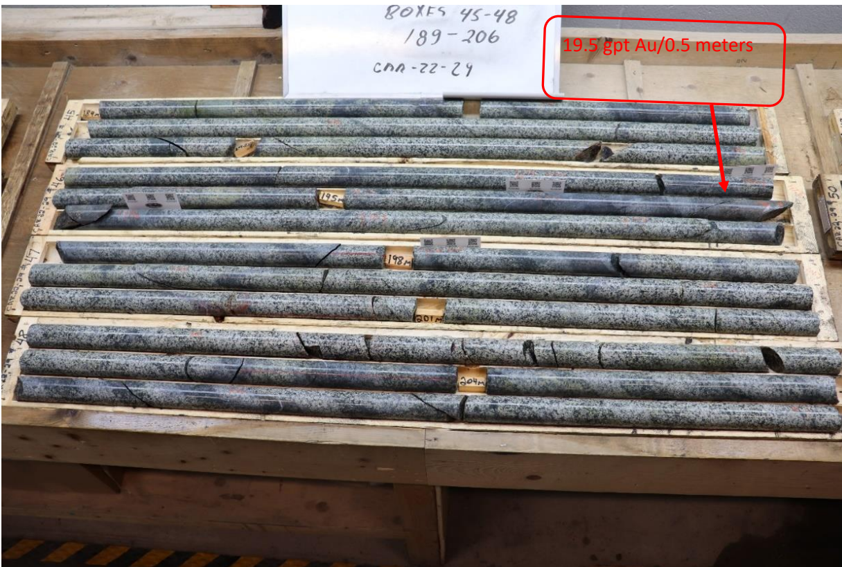
Figure 8: Drill core intercept in CAR-22-29 in the 1010 North Zone showing sulphidic vein within carbonatized granodiorite.
