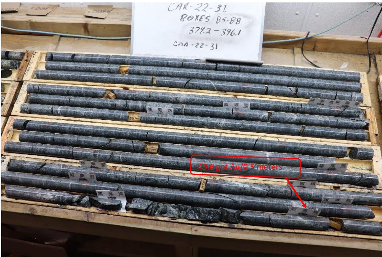
Figure 9: Drill core intercept in CAR-22-31 showing sulphide vein within carbonatized granodiorite.
