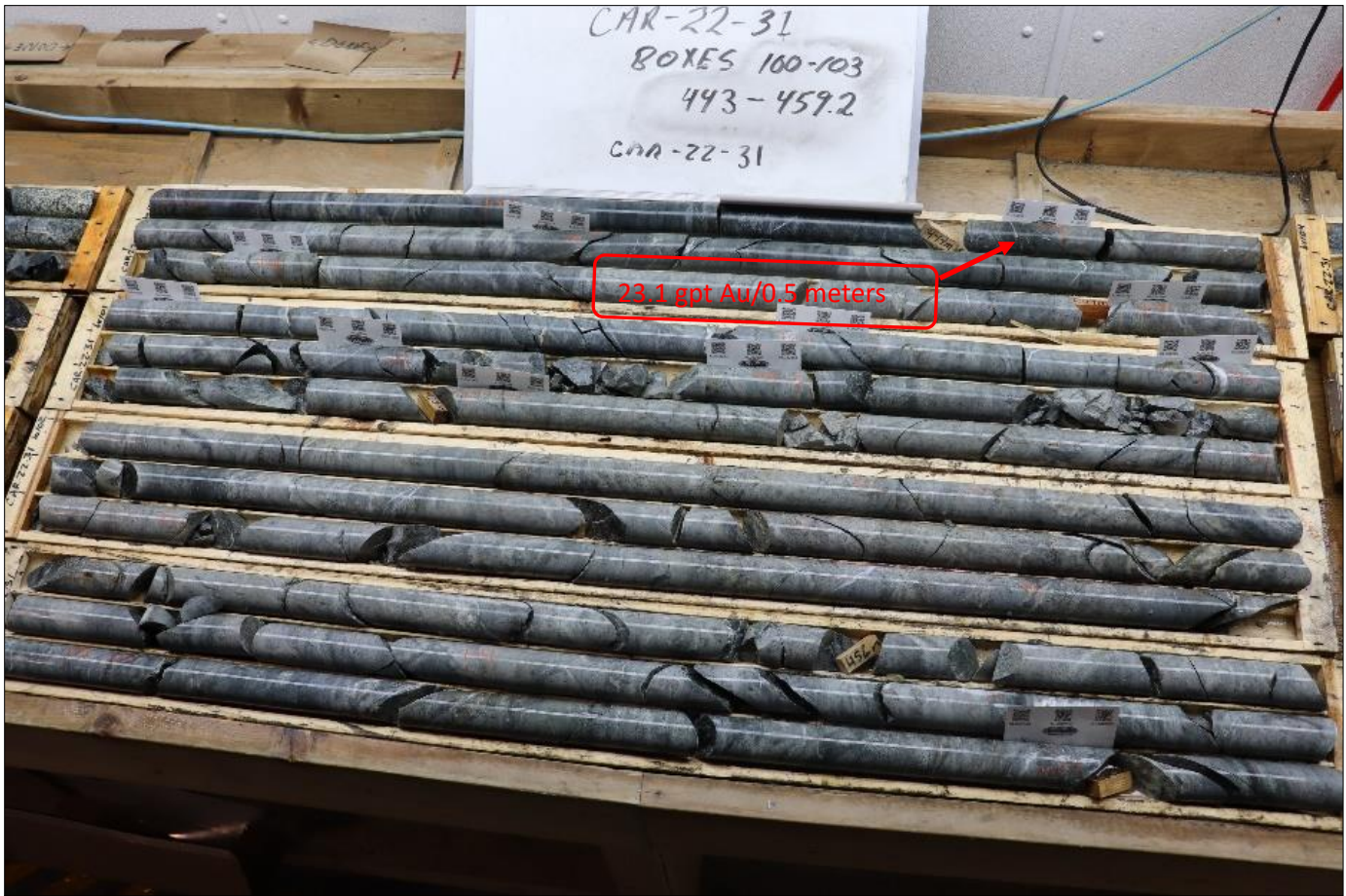
Figure 10: Drill core intercept in CAR-22-31 showing quartz sulphide vein (po,py,cpy) within magnetite-rich iron formation.
