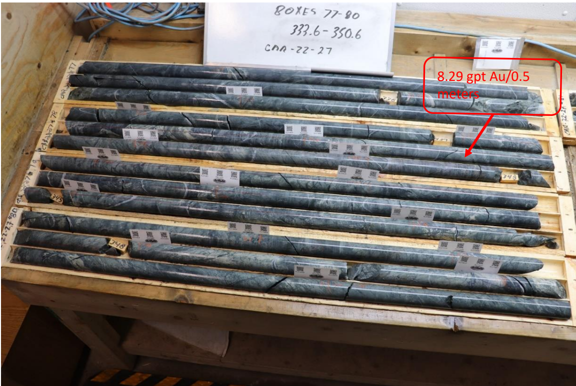
Figure 7: Drill core intercept in CAR-22-27 showing quartz sulphide vein (po,py,cpy) within mafic flow breccia.
