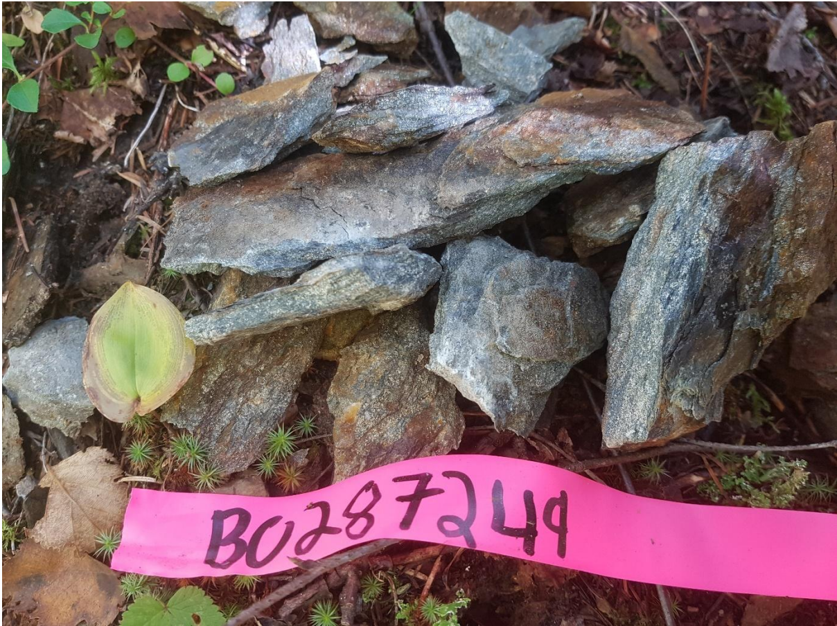
Figure 10: 15-20% pyrite in gossanous rock in the trench off the highway a little.
