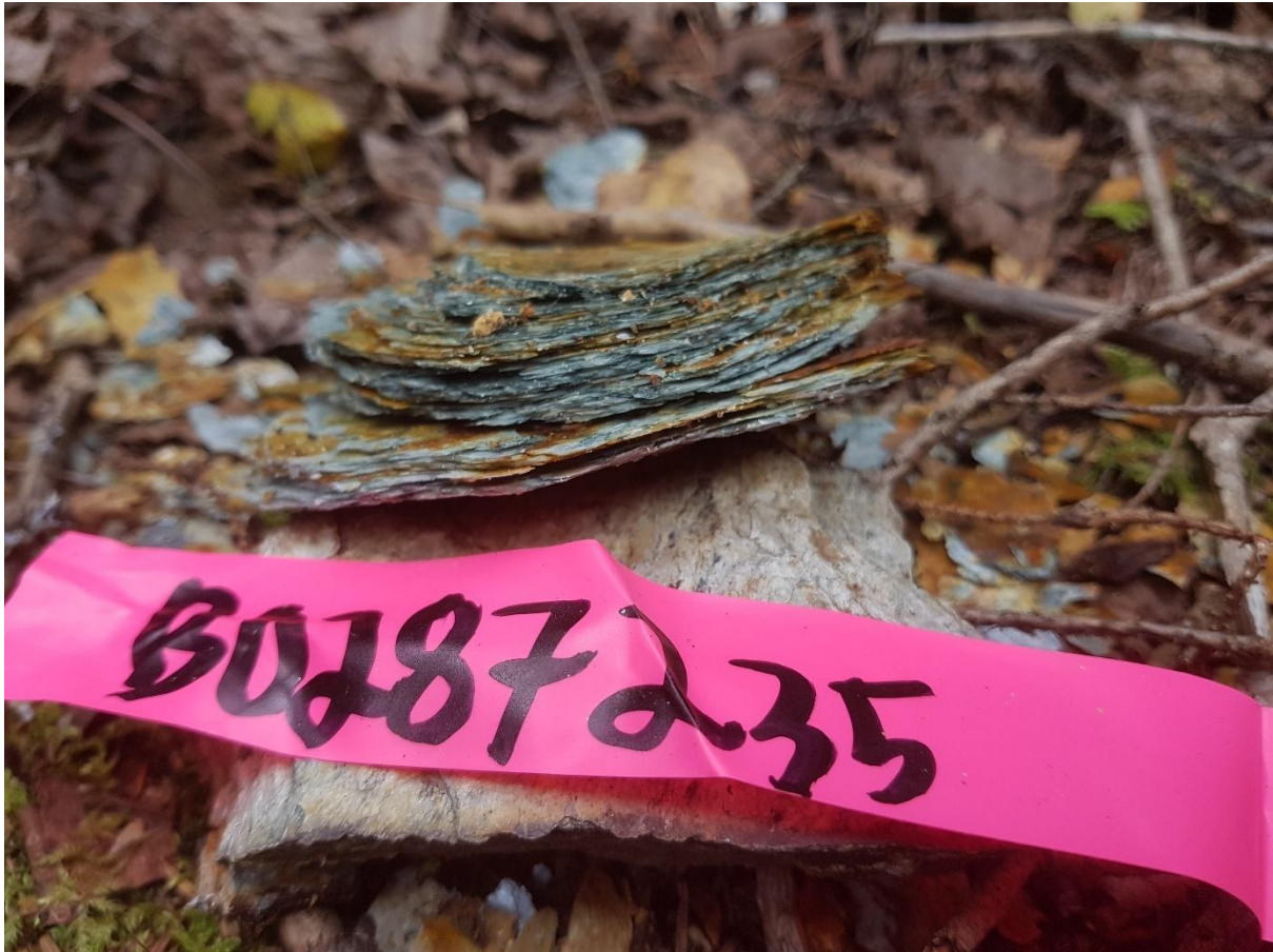
Figure 8: sericite schist with veined and disseminated pyrite in old trench parallel to GSH-11-01
