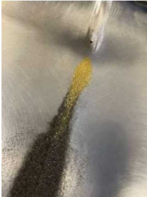
Figure 1: Gravity Concentrate on Mozley Table
