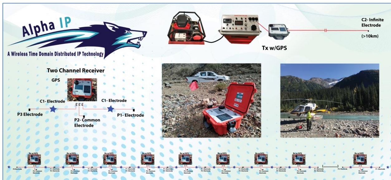
Figure 3-2: Alpha IP Schematic Spread Setup with Current Injection Offset.
