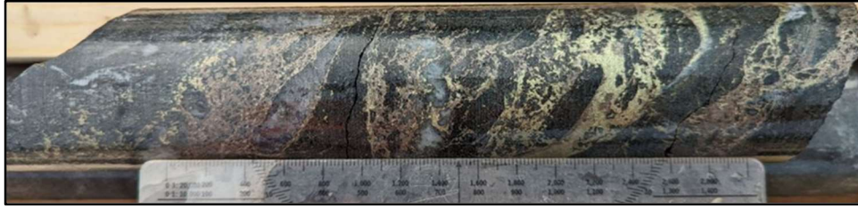
Figure 36. Mineralized sulphide breccia with pyrrhotite, chalcopyrite, and pyrite in hornblende gabbro at a depth of 46.00 m in QTBL0019.
