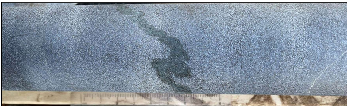
Figure 18. One centimetre-wide mafic band folded in biotite schist in QTBL0010 at 111.15 m depth.
