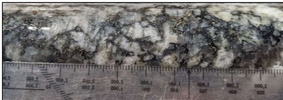
Figure 27. Weakly mineralized tonalite at 206.16 m depth in QTBL0013 with 2% interstitial pyrrhotite and chalcopyrite.
