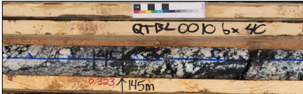
Figure 20. Brecciated diorite dominated by clasts of plagioclase feldspar in a biotite-chlorite matrix
