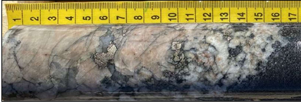
Figure 43. Patchy to interstitial pyrrhotite and pyrite mineralization in a pegmatitic granite at 25.00 m depth in QTBL0021.
