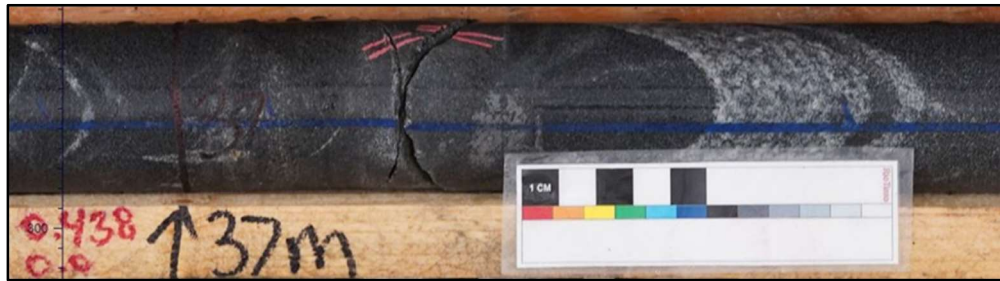
Figure 39. Felsic bands in fine-grained biotite schist at a depth of 37m in QTBL0020.
