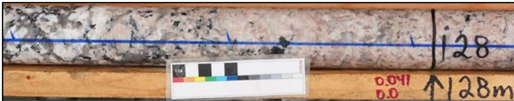
Figure 40. Variably textured granite units in QTBL0020 at a depth of 128m. K-feldspar and plagioclase content varies as well as grain size and biotite occurrence.
