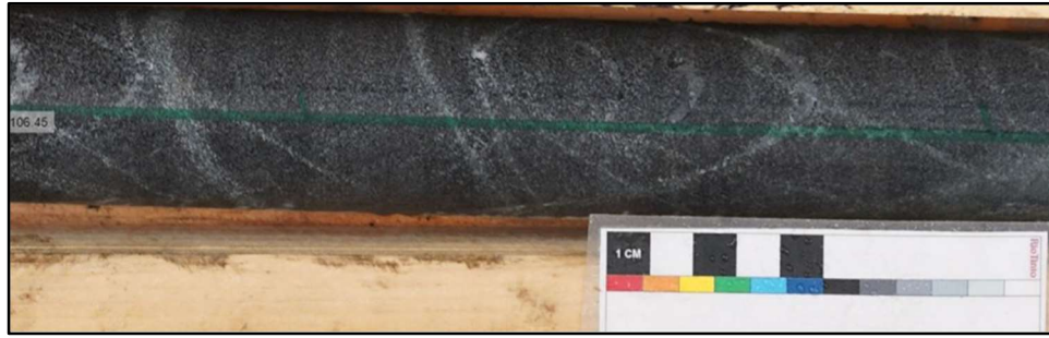
Figure 30. Biotite schist with multiple orientation of carbonate veins. Note chlorite vein halos around the carbonate veins.
