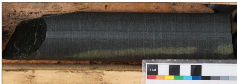
Figure 31. Diabase unit at 30.60 m depth in QTBL0017. Weakly disseminated pyrrhotite is present in the diabase.
