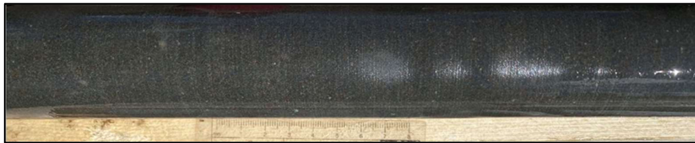
Figure 21. Diabase unit in QTBL0011 at 30m depth. Note the very fine disseminations of rusted pyrrhotite.
