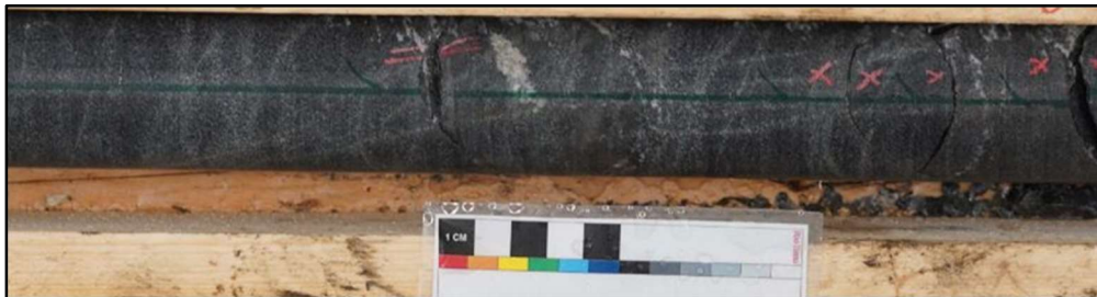
Figure 23. Biotite schist country rock with carbonate veining and common felsic boudins. 25.5m depth in QTBL0012
