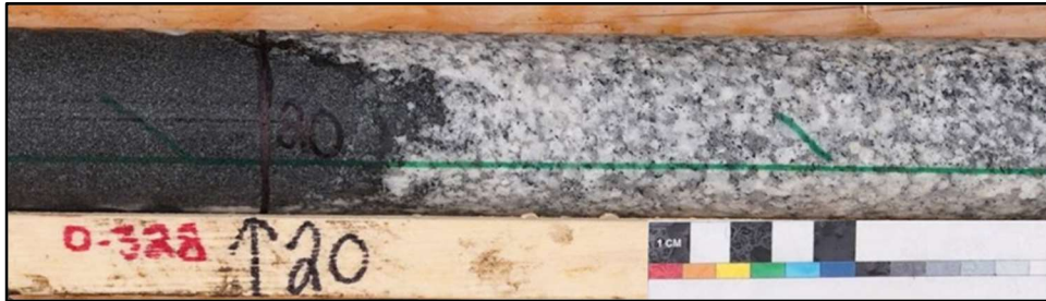
Figure 28. Biotite schist contact with a medium-grained bleached granite at 20m depth in QTBL0014
