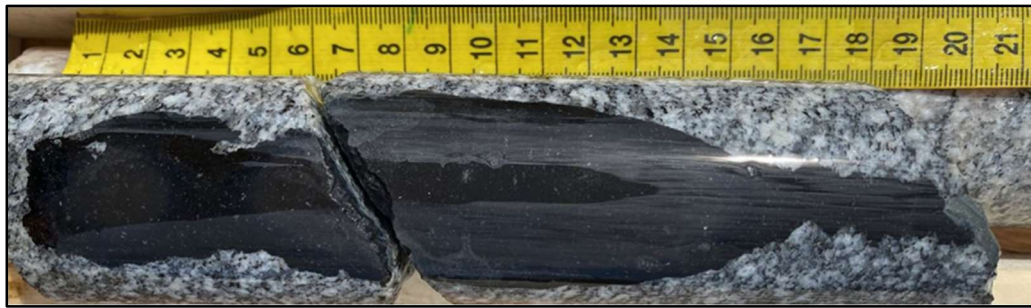
Figure 44. Diabase occurring in quartz diorite unit in QTBL0021. Diabase hosts 1% patchy pyrrhotite mineralization.
