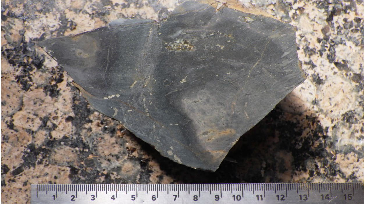
Figure 13. Sawed hand specimen of mineralized silicified basalt from waypoint SC2 (metric scale in centimetres).
