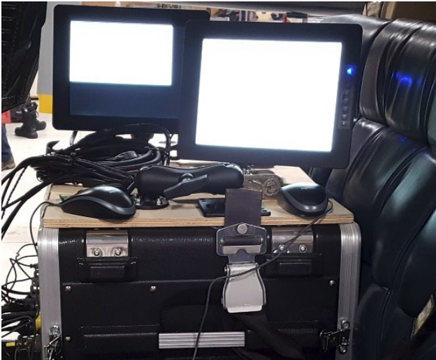
Figure 3 – EGL Navigation Computer, Moving-map Display
