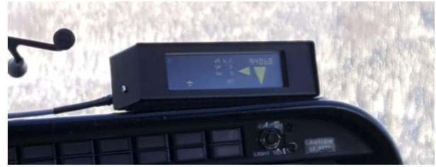
Figure 4 – Pilot Steering Indicator and Radio Altimeter Indicator
