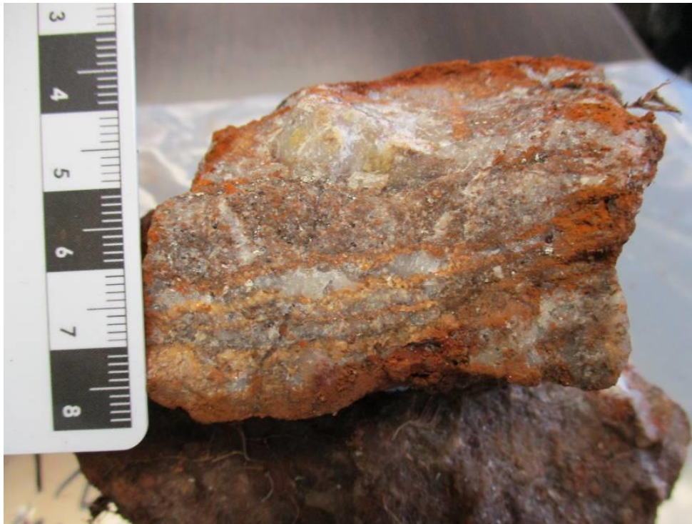
Plate 1: strong carbonate alteration with quartz veinlets and disseminated pyrite: 3.84g/t Au (BLS23-10)
