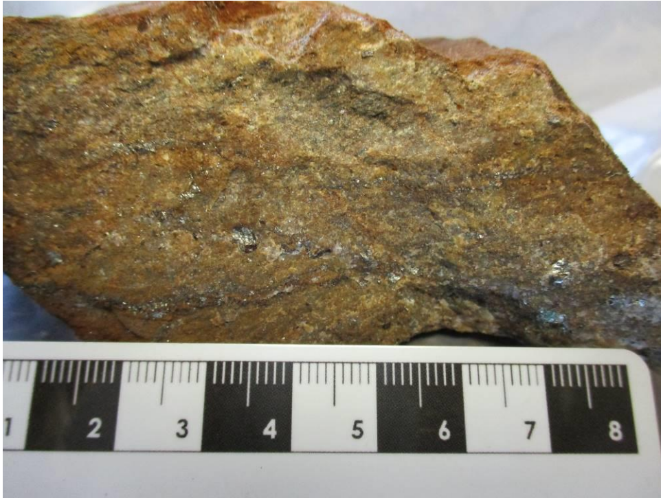
Plate 2: strong carbonate alteration with weak stringer and disseminated pyrite: 11.40g/t Au (BLS23-13)
