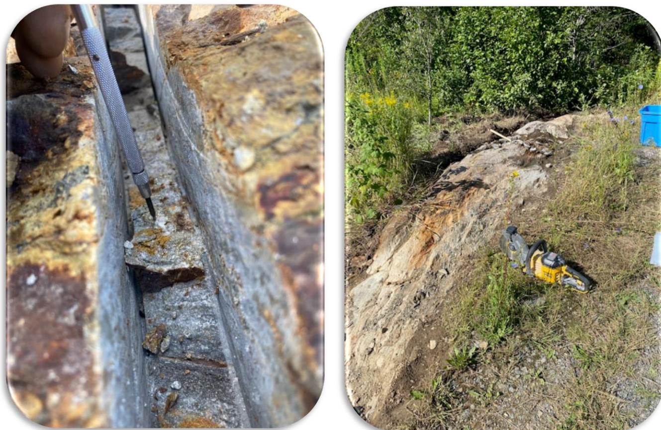
Figure 8 - close up view of channel cut in sheared and sulfide mineralized intermediate volcanics (left) from hand stripped and reclaimed outcrop (right)
