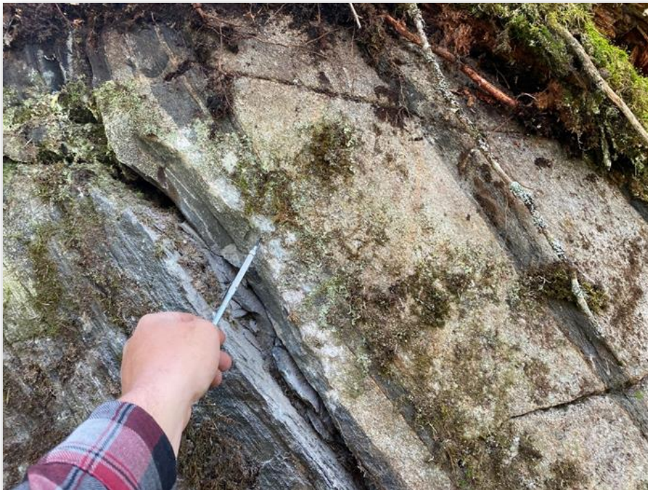
Figure 6 - QFP dyke intrudes thinly bedded sediments.
