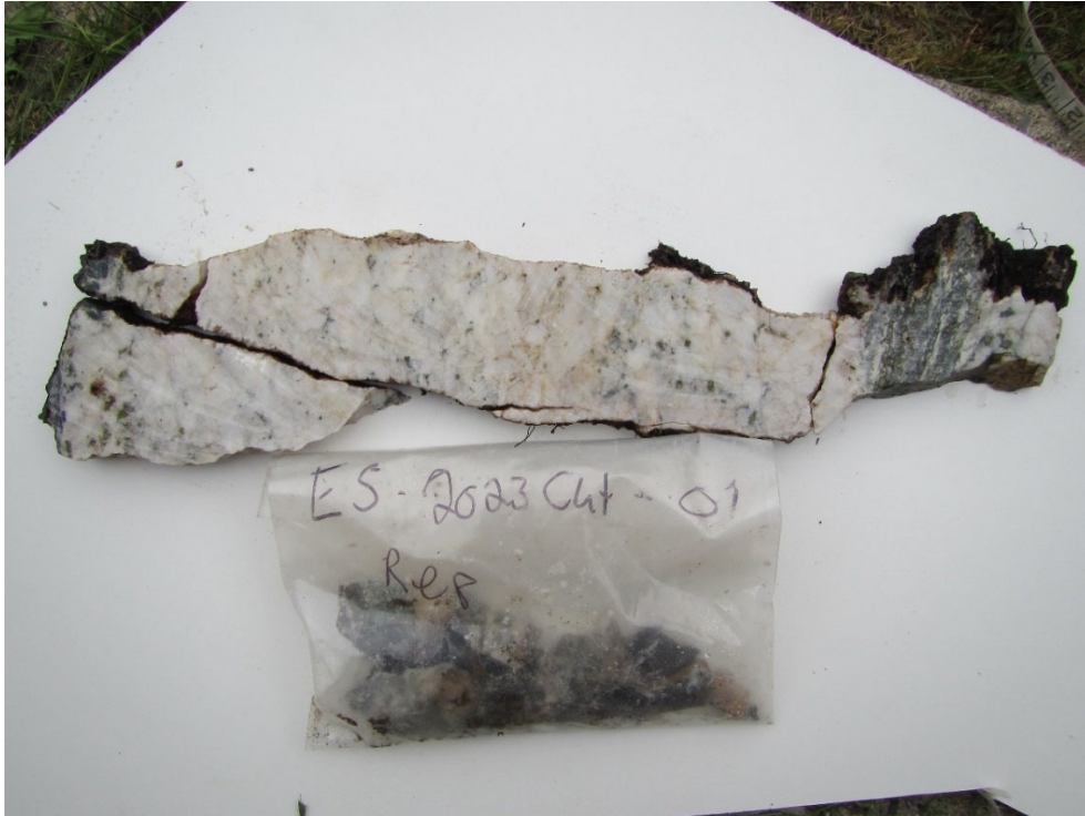
ES-2023Cut-01Rep, 50cm long, blebs of Cpy throughout. Picture of rep provided as second cut didn't break as much during extraction. Mineralization in both cuts very similar.
