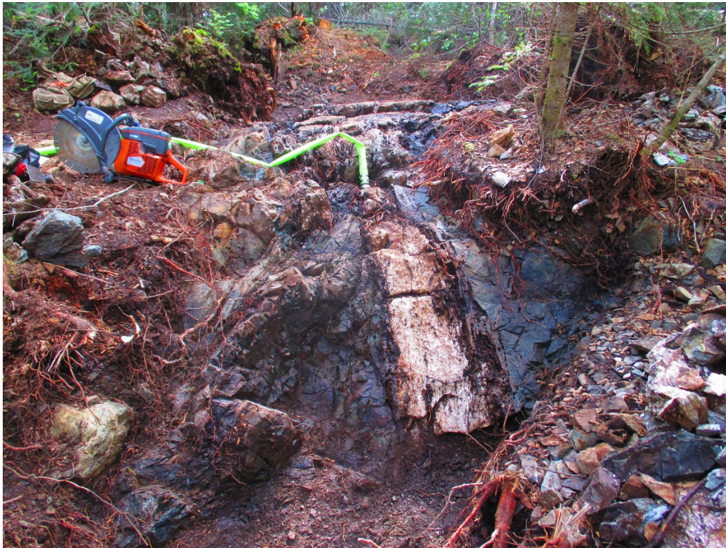
Main BenoMath vien – looking east, 40-50cm wide quartz Cpy vein, steeply/near vertical dipping, heavily fractured/faulted dark blue host rock, picture taken during channel sampling June 2, 2023
