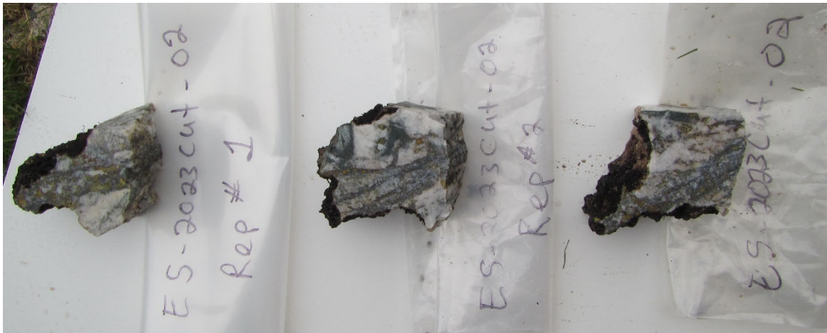
ES-2023CUT-02 carbonated quarts with chalcopryite blebs, brecciated host rock within veins, multiple reps taken with slight variation in each.
