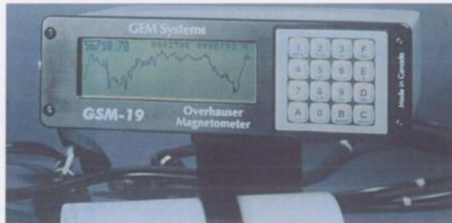
Overhauser (GSM-19) console with sensor and cable. Can also be configured with additional sensor for gradiometer (simultaneous) readings.
