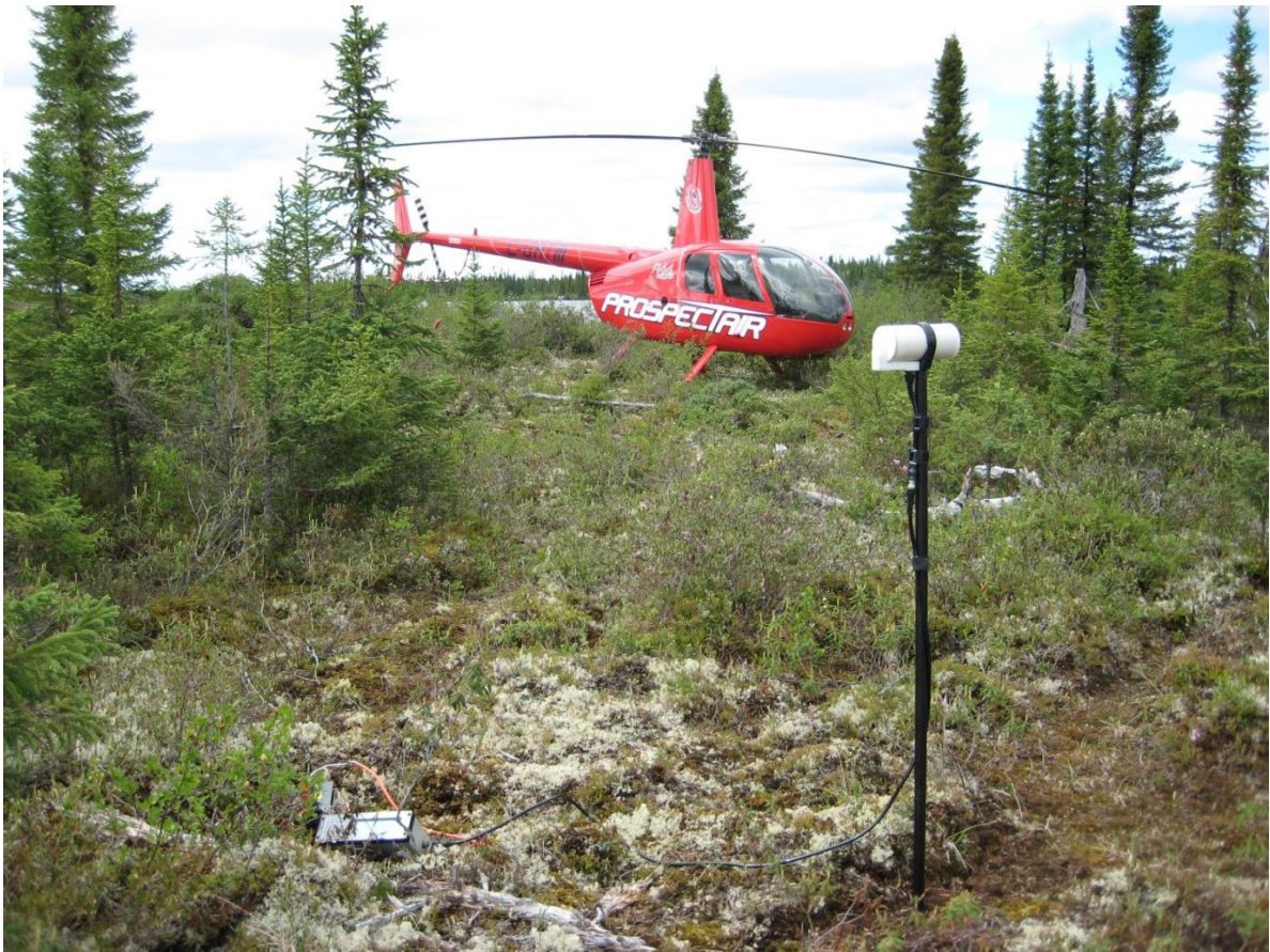
Figure 8: Example of a magnetic base station setup
