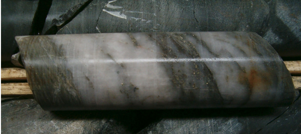
Figure 8. Laminated quartz-biotite-chlorite crack and seal vein with 5% disseminated pyrite from EMP08-02 at 110m depth.
