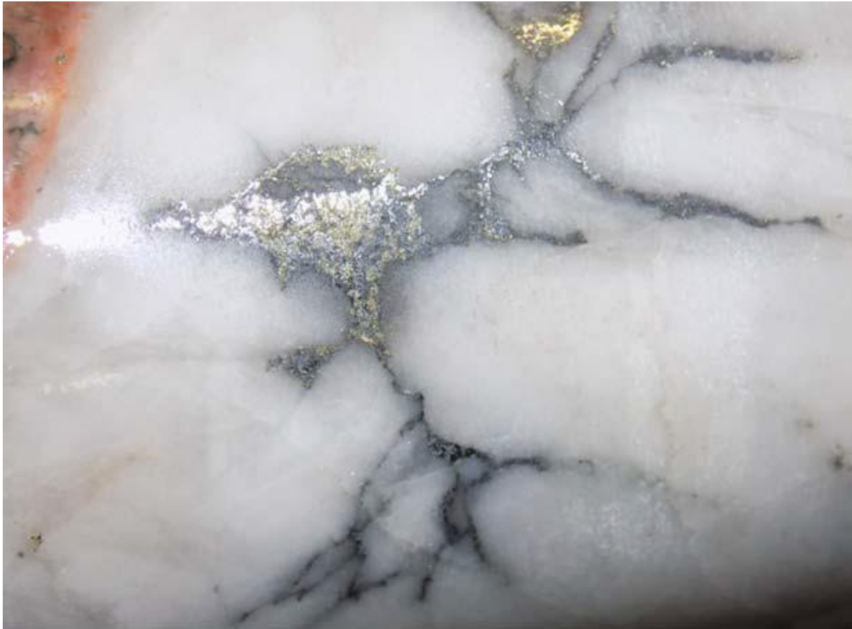
Figure 5-3 : Au-Bi-Te stringers in quartz vein from 54.6 m, MG-14-12.
