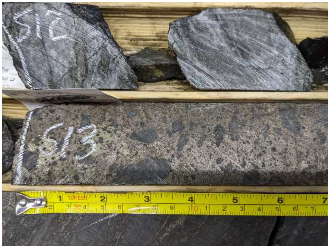
Figure 5 Hole CALD-22-01 Sulphide Zone, close-up of pyrrhotite at 337 m.
