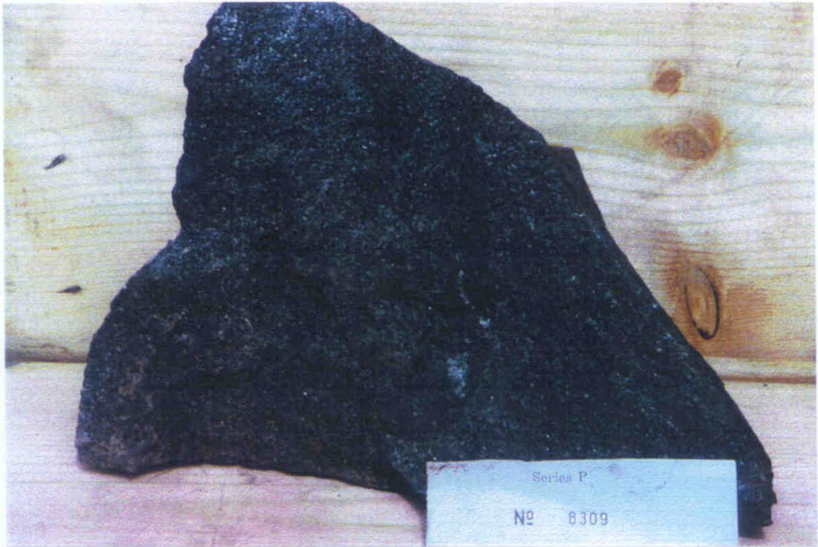
Photograph: 19 (Above) Diabase sample 8309 from Central Outcrop at 16+620.
