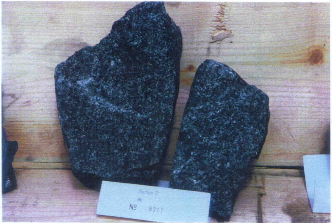
Photograph: 23 (Above) Diabase sample 8311 from South Outcrop at 16+458.
