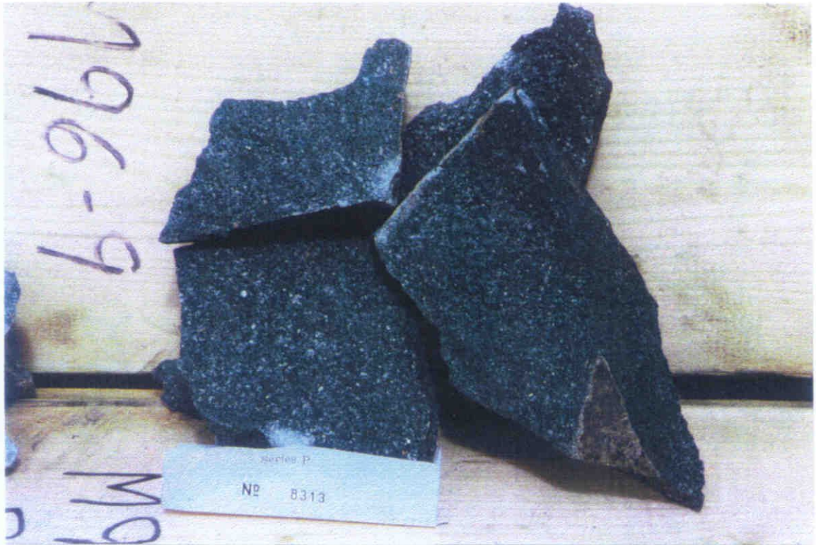
Photograph: 27 (Above) Diabase sample 8313, Roosevelt Road Quarry Site #1, 2.4 km east of Highway 11. Photograph: 28 (Below) Close up of sample 8313.
