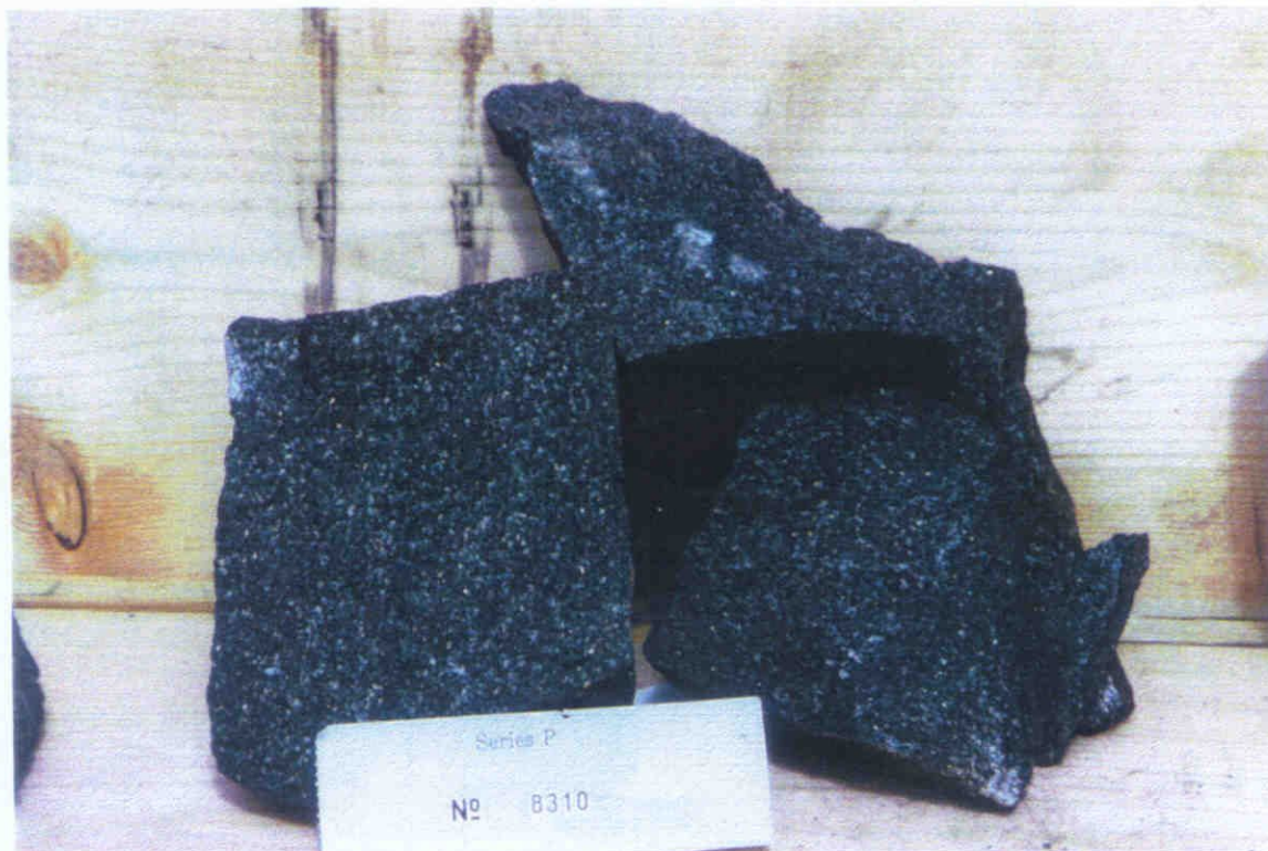
Photograph: 21 (Above) Diabase sample 8310 from Central Outcrop at 16+730.
