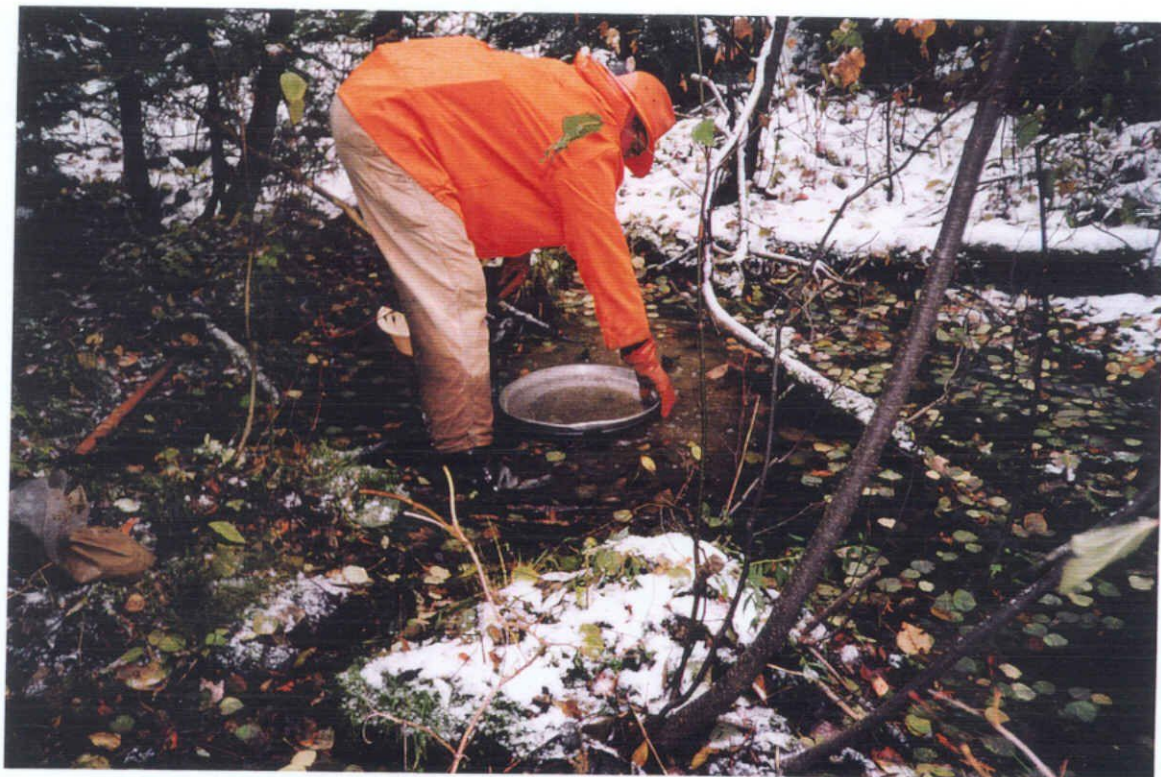
Preliminary screening of till samples, K-7, K-8 and K-9 in melt water in field.
