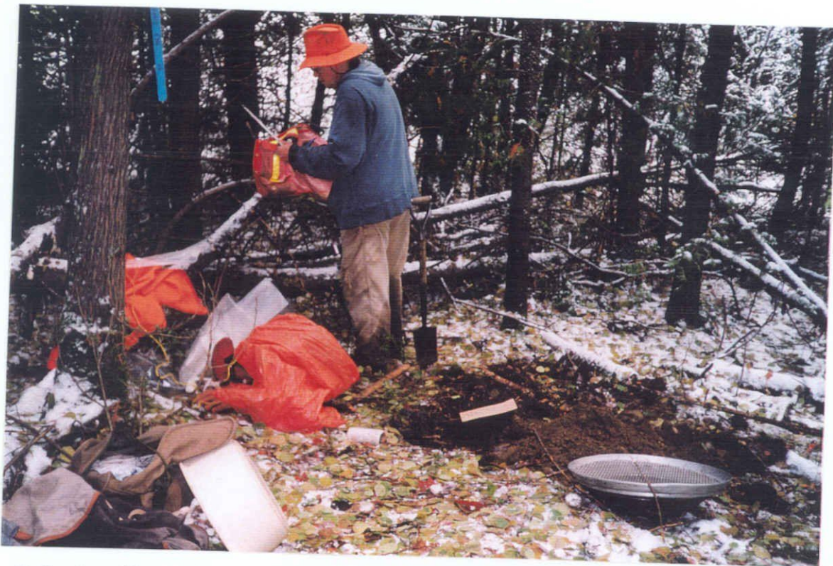
Collecting till sample on Keating Anomaly. Sample pre-screened over sized materials
