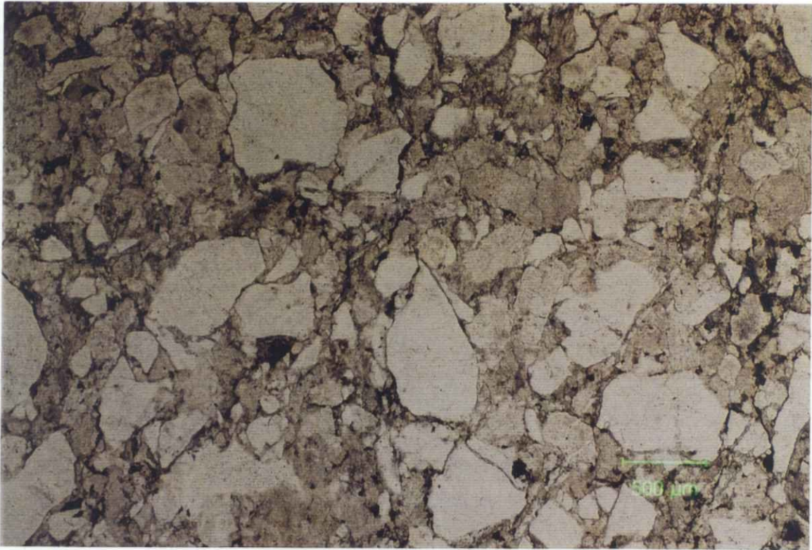
Figure 17. Arkose in plane-polarized light. Sample NL-73
