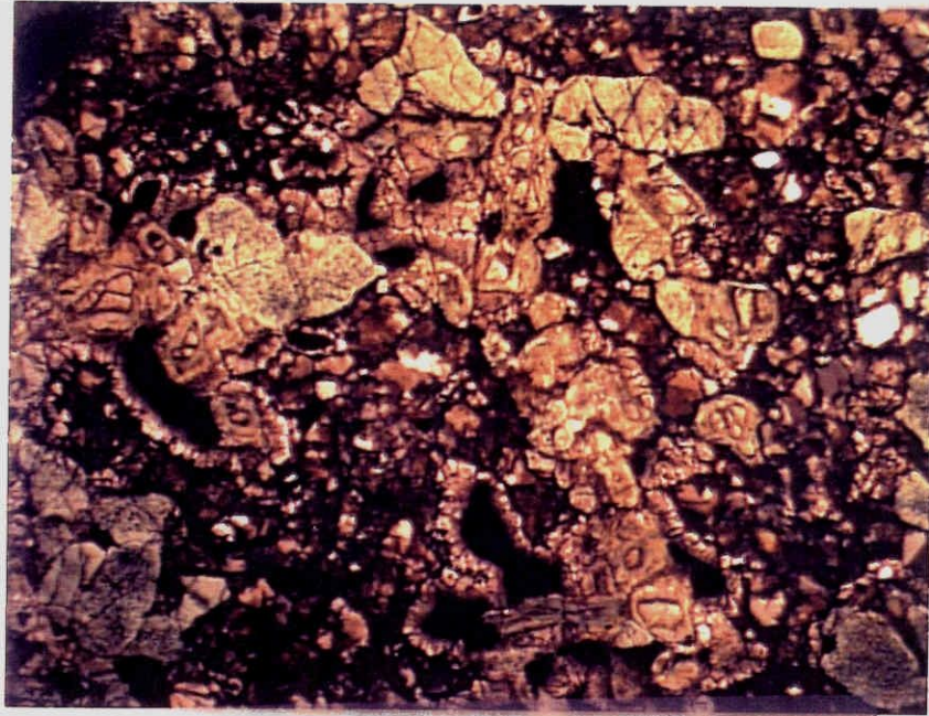
Fig. 16. Highly altered, pyroxene (light green) - plagioclase (dark brown) rock with subsolidus reaction garnet (pinkish). Sample #8 (FOV 7 mm PPL).
