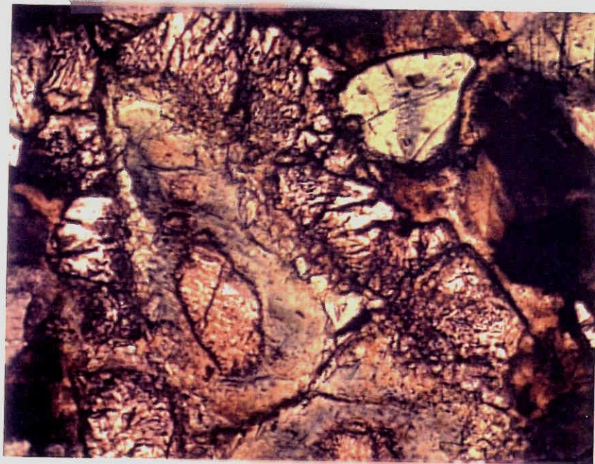
Fig. 17. Light green diopside mantled by, and intergrown with, colourless-to-pinkish, fluid inclusion filled-garnet. Sample #8. (FOV 4 mm PPL).
