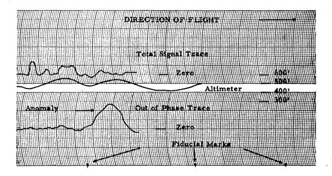
The bottom trace is a record of the Out-of-Phase component. Its zero position is in the centre of the chart. Anomalous peaks are always positive, i.e., they rise above the zero position. Negative peaks have no direct significance. Peaks marked S are calibration markers.
