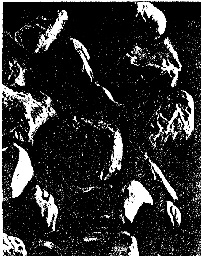
Fig. 4. A gold blade (particle 16), which probably is an elongated gold crystal. 450X.
