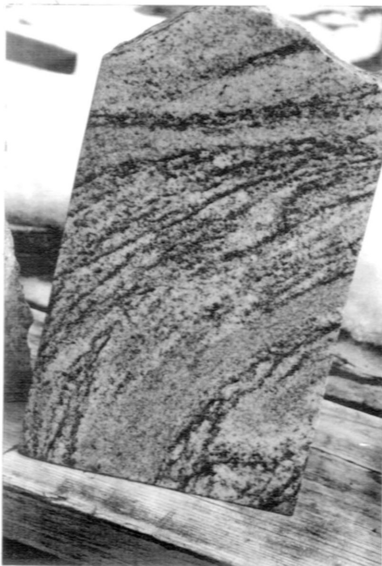
Photo 1 Migmatite Outcrop(above) and Photo 2 Polished Migmatite (below) Black Lake depicting the pink-mauve and buff and grey variegated, veined migmatite in outcrop and polished slab respectively. The rock takes a very attractive polish. The intense red is caused by extremely fine hematite staining. The basic colours are amazingly similar to those existing on the other properties which are 20 miles to the south.
