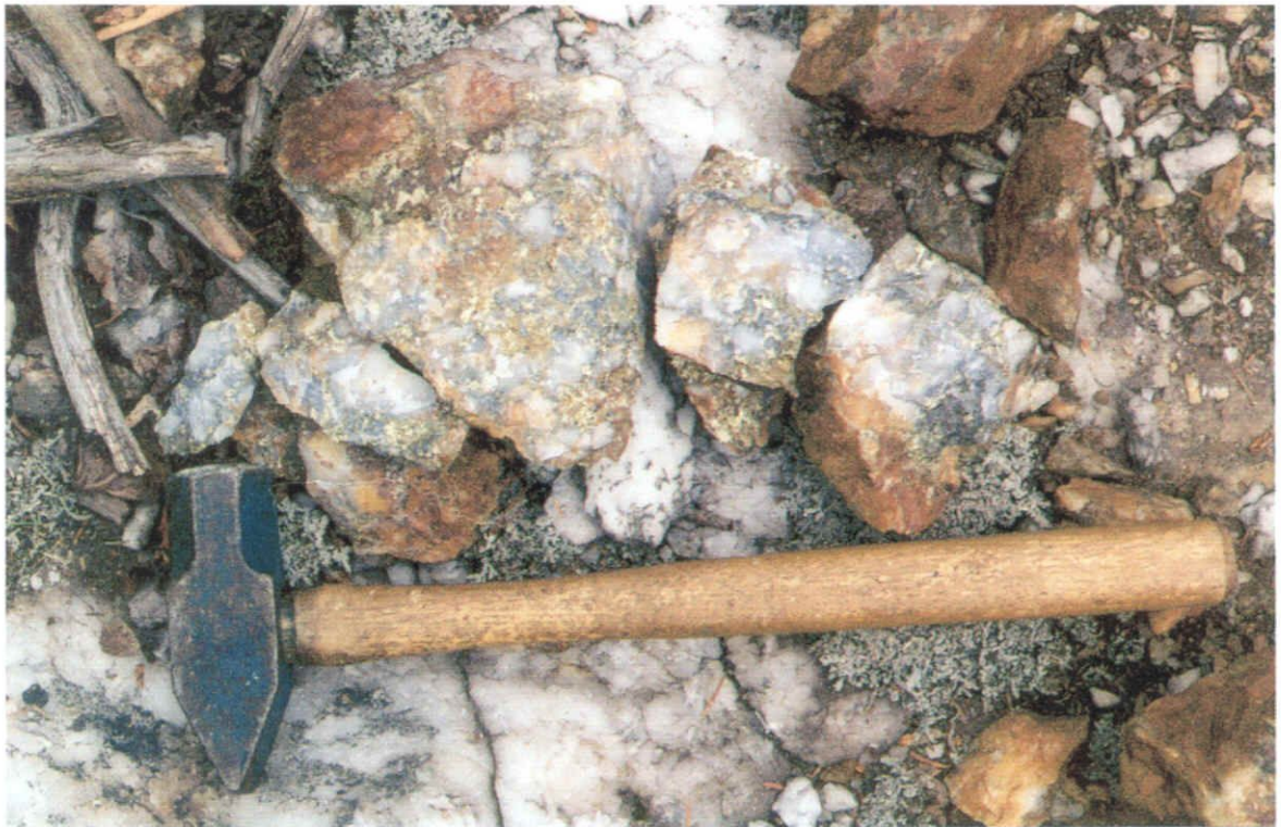
Chalcopyrite, quartz vein breccia, deformation zone, L2W/3S
