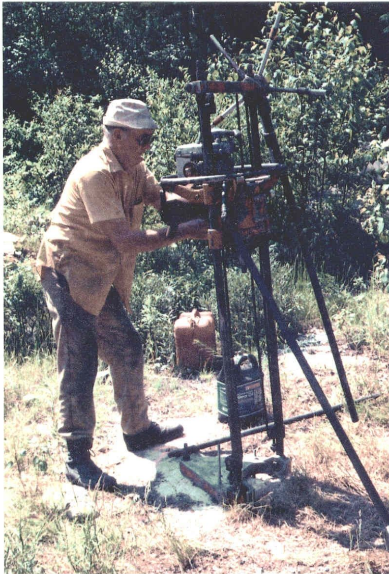
Angus Macdonnell, Contractor, Setting Up At DDH 95-1 . This Hole Was Abandoned Short Of The Target Because Of Very Hard Rock.
