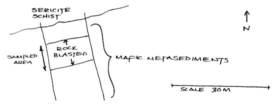
410 LBS TAKEN AND CRUSHED TO -3/8". 4.1 LBS TAKEN VIA MECHANICAL SAMPLER 4.1 LBS SENT FOR ASSAY - SAMPLE #15883
