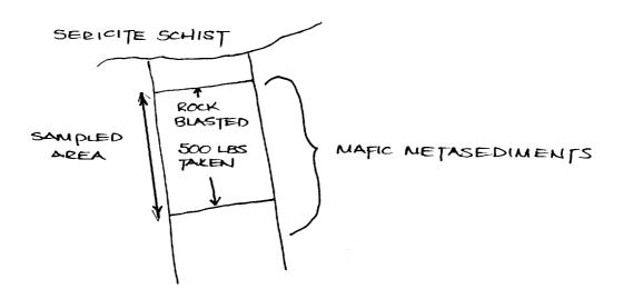
500 LBS BULK SAMPLE CRUSHED TO -3/8"
