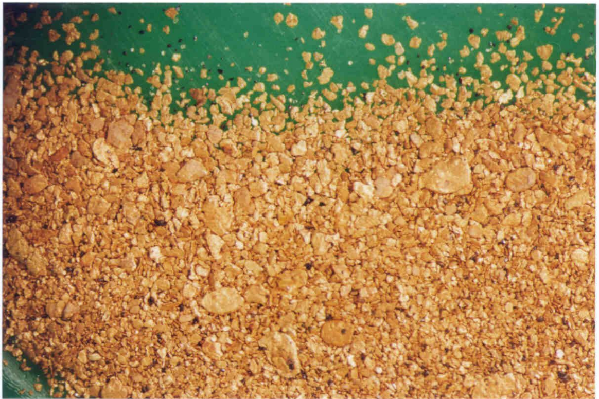
[ii] Gold grains at 28 times magnification with the largest grain at approximately 1.5 mm x 1mm in size. Larger sized gold grains would of been discarded with waste material during sieving and panning. Screen mesh size was 1/20 th of an inch.
