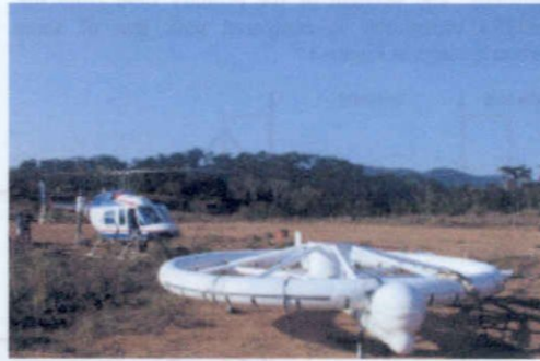
Figure 1. The AeroTEM airborne electromagnetic system.
