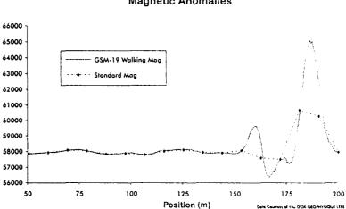
As shown above, near-continuous measurements increase definition. Results from a GSM-19 "Walking Mag" (273 readings over 150 m with 2 sec. cycle time) were compared with results from a standard magnetometer (13 readings over 150m).
