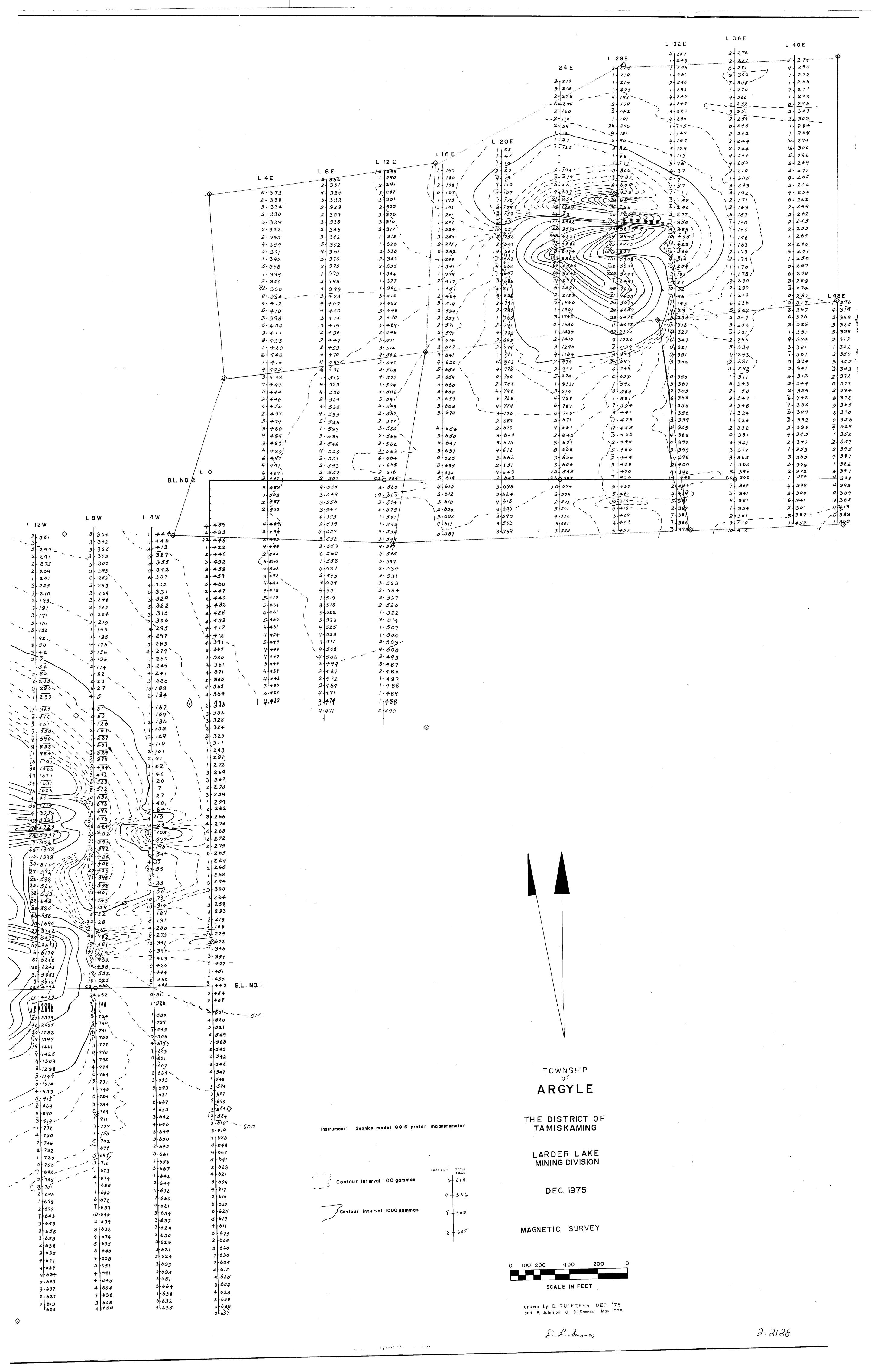
L 40E L 4E' 25 B 2211236767676767676767677767777 ELECTROMAGNETIC DATA obtained by using A RONKA EM.16 instrument - OPERATOR FACING NORTH USING MAA CUTLER, MAINE FREQUENCY: 17.8 kHz. IN PHASE OUT-OF-PHASE POSITIVE VALUES
