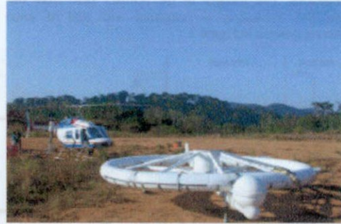
Figure 1. The AeroTEM airborne electromagnetic system.
