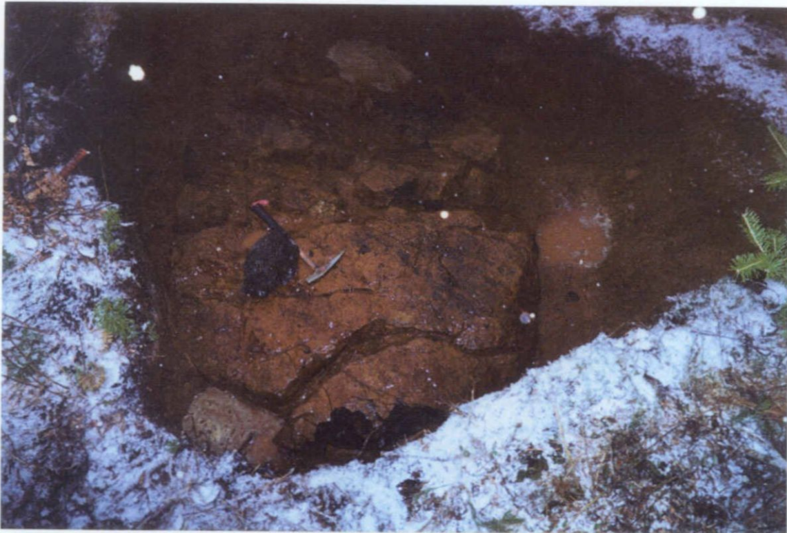
Pit of samples 111-113 of conductor trending 130 degrees. Ultramafic locally contains 15% fine-grained magnetic pyrrhotite cumulates.
