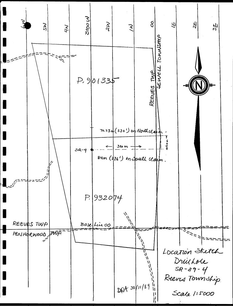
.0 .0 DIAMOND DRILL RECORD HOLE NO. : SR.89-4 360.0 Azimuth: Section: L3+00W **Property:** SEWELL-REEVES Dip: -50.0 Core Size: BQ Location: L3+00W 3+60N Elevation: .0 Date Started: September 28, 1989 154.2 Length: Date Completed: October 4, 1989 D. Alexander Logged by:
