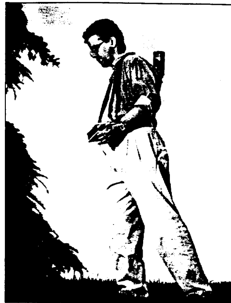
ENVI-MAG Proton Magnetometer in operation
