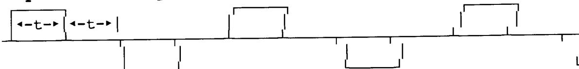
$t = 2$  seconds, ON & OFF time. Total duty Cycle Used; 8 seconds.
